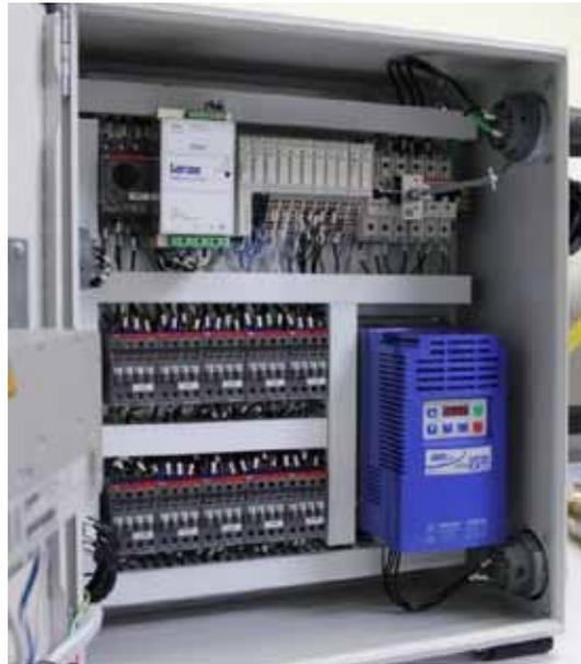
Right: IP65 Enclosure provides protection from dust, oil and water wash down. Electronics meets UL-508C standards for Industrial Control Equipment. The system is completely controlled via an easy to use touch screen and can also be controlled remotely via the Internet.
